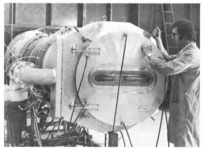
EXPERIMENTS with lasers pumped by electron beams are the primary use planned for this 20 kilojoule electron beam machine now being installed in the new laser physics laboratories in Bldg. 893. Built to Sandia specifications, the machine's maximum output will be two million volts at 200,000 amps for 50 nanoseconds. John Bagg (5212), project leader, expects the machine to be operational by the first of the year.
